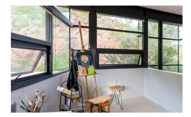
The **Series 670 Awning Window** from Western Window Systems hinges on the top, opens outward, and is typically wider than it is tall. Ideal for providing natural light and ventilation to small areas, it saves space by opening out from the bottom.
