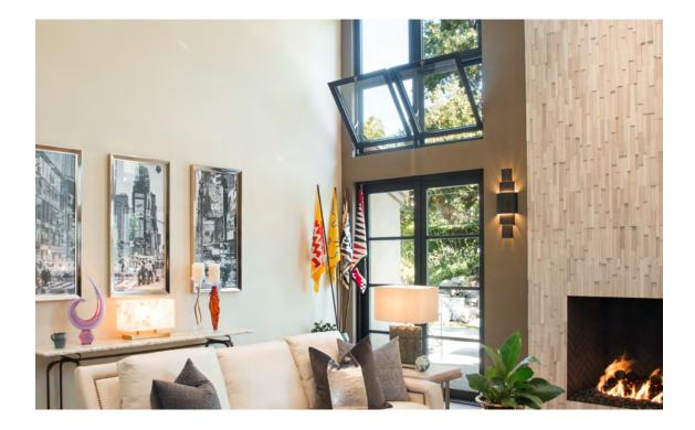
Perfect for places where there is limited space for a window to extend to the outside, the Series 7680 Hopper Window hinges on the bottom and opens from the top.
