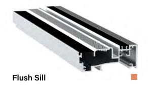
When ease of entry is more important than climate performance, the flush sill lines up with most interior flooring for a smooth transition to the outdoors. Interior threshold height is 1.76". Thresholds are finished to match the color of the frame.
