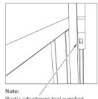
Plastic adjustment tool supplied. Tip to be removed after final adjustment.
