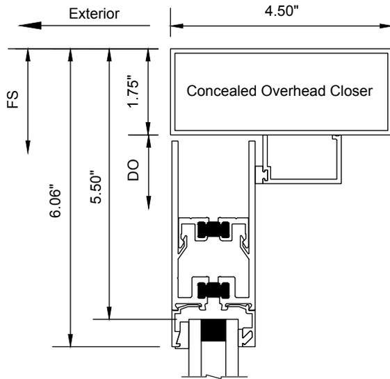
Series 900 Hinged Door - Swing Out - Medium Stile - Thermally Broken - Concealed Overhead Closer - Equal Leg Block Frame
