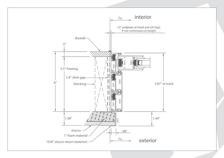
*Note:* Be certain to seal the back side of the applied corner sections at the top of each jamb extending a minimum of 3" in each direction to ensure a weather tight seal. (See Diagram). Follow all directions to finish the installation.
