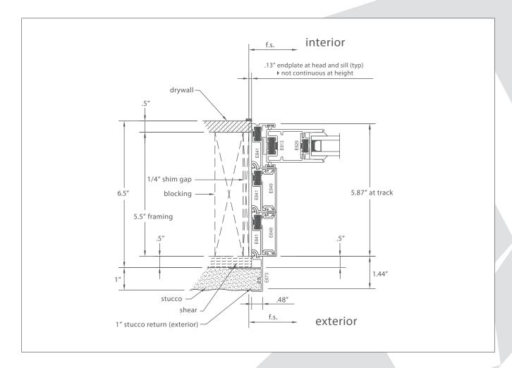
The intended use of this optional kit is to provide a return surface to aid in the installation process, waterproofing, and to create a solid return for stucco or other exterior finish applications. This return is designed to work only with Series 600 non-pocket multi-slide doors from Western Window Systems. Due to field conditions, 90-degree corner units are excluded from this kit option.
